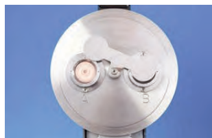
Dual sputtering heads and automatic shutter
