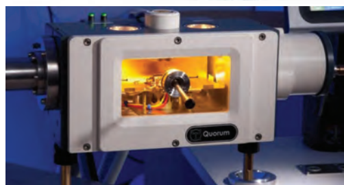
Cryo preparation chamber with cryo transfer device fitted
