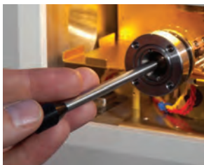
Front-mounted fracturing and specimen manipulation tool
