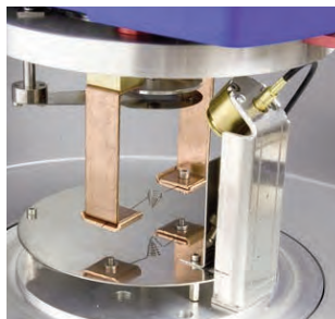
Metal evaporation insert (set up for upwards evaporation)
