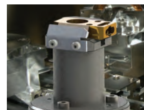
QuickLok specimen stage and adaptor to SEM
