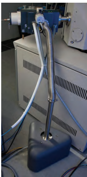
Remotely mounted turbomolecular pumping system
