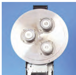
Triple sputtering head with automatic shutter open
