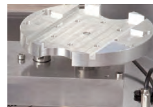
Specimen stage for glass microscope slides (option)
