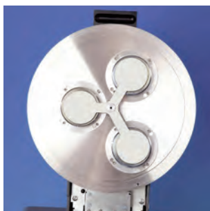
Triple sputtering head with automatic shutter closed
