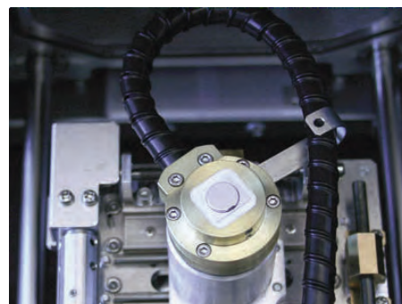
Standard Coolstage. Range: -30°C to +50°C at 300Pa
