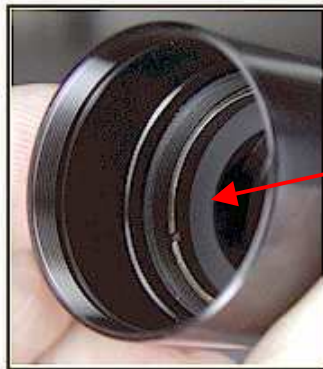
Position of reticle in Kelner type eyepiece
