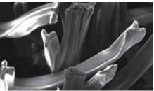
Au Sputter Coat Magnification : x500 Os PE-CVD Coating provides a great Au Sputter Coating is an anisotropic, directional coating process. It does not imaging without losing the original sur- fully wrap around the sample which can face texture. The different appearence cause charging effects in some areas. The
