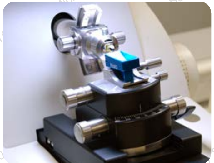
Chuck attached to microtome.
