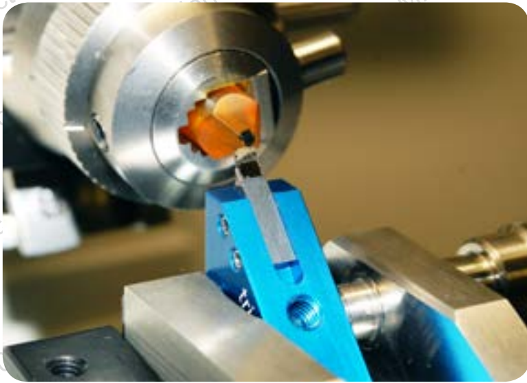
Trimming block face with a using a Diatome trim tool.
