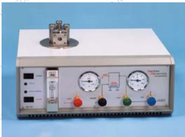
EMS Q850, critical point dryer.
