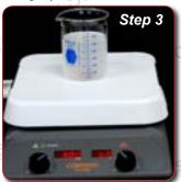
3. When the water and buffer solution reach 60°C, turn off the fume hood and 1 gram of paraformaldehyde to the heated solution, wait until it goes into solution and continue with the next gram and follow this routine until all of the paraformaldehyde is in solution. BE SURE to turn the fume hood back on.
