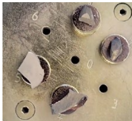
Ceramic samples after coating
