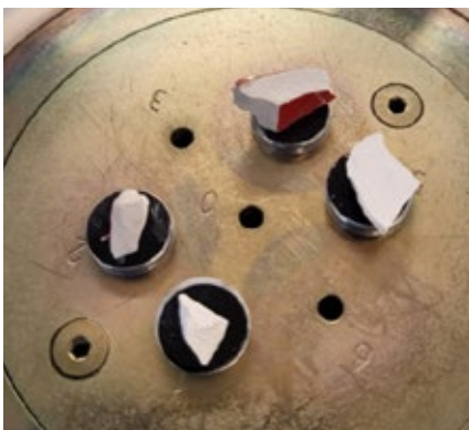
Ceramic samples before coating
