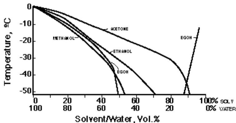
Graph 1: Freezing points of commonly used dehydrating agents (solvents) as a function of concentration. EGOH + Ethylene glycol. Note the rise in the freezing point of EGOH at higher concentrations.
