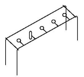
Fig. 1. A wire capsule holder for UV polymerization.
