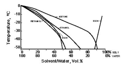
Graph 1: Freezing points of commonly used dehydrating agents (solvents) as a function of concentration. EGOH + Ethylene gylcol. Note the rise in the freezing point of EGOH at higher concentrations.
