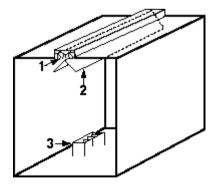
Fig 2. A polymerization chamber for indirect UV irradiation, the UV source (1) is diffused by a right-angle reflector (2). The capsule holder (3) is place 30-40 cm below the UV source. See section 5.1
