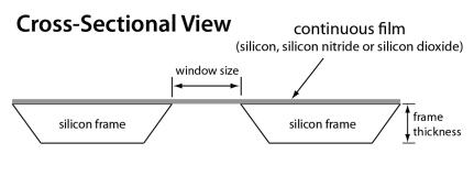
TEM and X-Ray Windows are packaged in silicone gel-boxes with their suspended membrane films facing up (see cross-section). The suspended membrane side of TEM and X-Ray Windows should never be placed onto another surface in the opposite "face-down" orientation.
