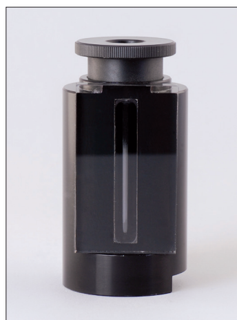
PGF Tube Holder for the SW60 or similar rotors
