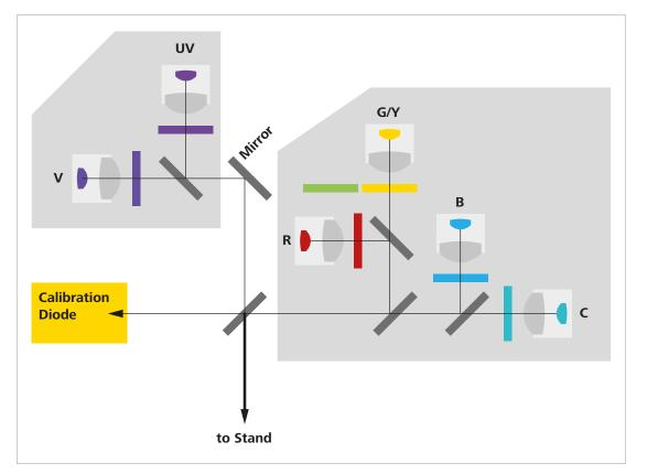
Schematic representation of 7-channel Colibri setup
