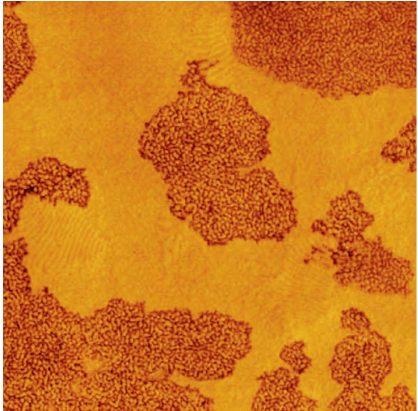
▲ Morphology of a blend of two SBS block copolymers with different chain-architecture. AFM tapping mode, phase image, image size = 3 x 3  $\mu\text{m}$ . Rameshwar Adhikari, Institut für Werkstoffwissenschaft, Martin-Luther-Universität, Halle-Wittenberg.
