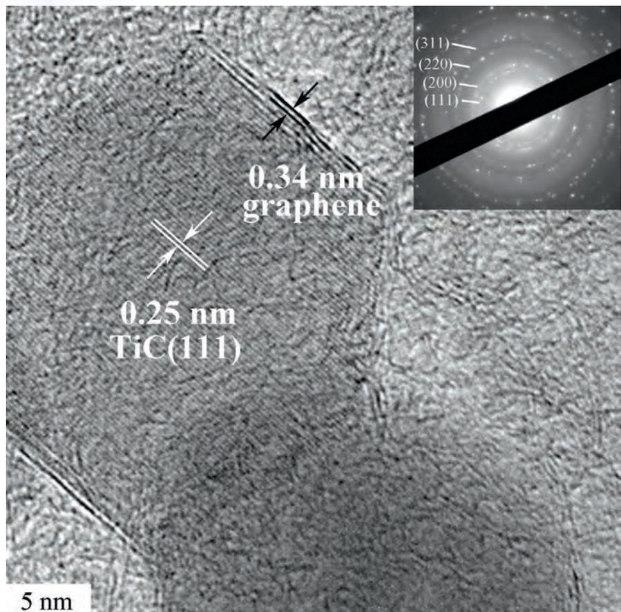
▲ HRTEM image of a TiC microsphere showing nanocrystalline carbon coating on the TiC grain (confirmed by the electron diffraction pattern).
