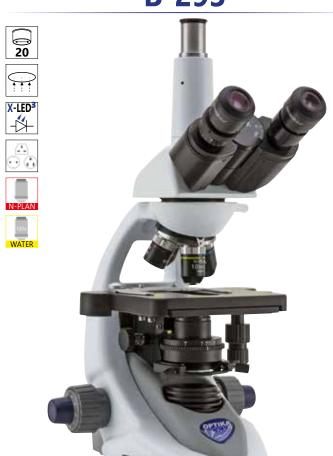
Trinocular head with N-PLAN objectives, rackless stage and exclusive **X-LED**<sup>3</sup> for unmatchable performance, powerful and uniform illumination.
